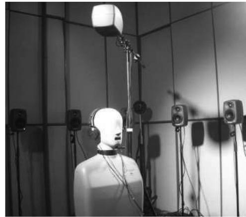
**Fig. 3** Setup to measure the passive attenuation for different directions of incident sound with loudspeakers around and above the test subject
