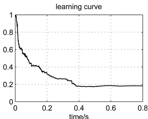
**Fig. 8** Learning curve of the LMS algorithm for the broadband aeroplane noise
