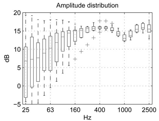
Fig. 7 Variation of  $S$  in third octave bands, for four users and a dummy head
