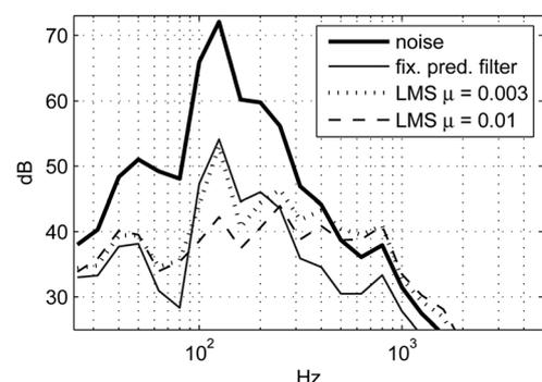
**Fig. 10** Engine noise  $x$  that entered the headphone and the residual noises after ANC
