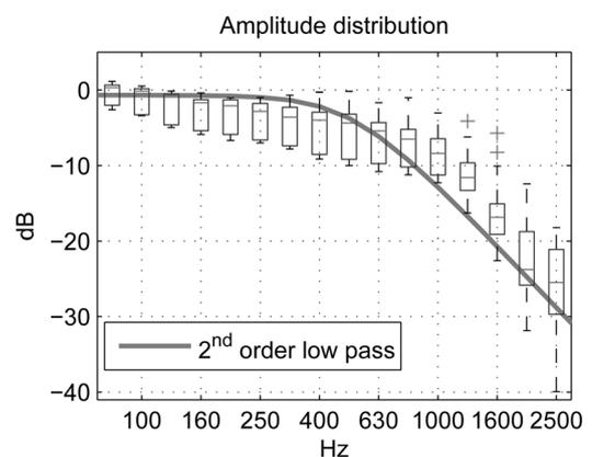
**Fig. 4** Variation of the passive attenuation in third octave bands for different users, different leakage situations and different directions of incident sound
