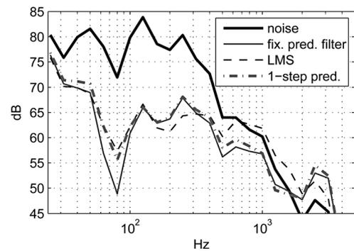
**Fig. 9** Spectrum of the aeroplane noise  $x$  that entered the headphone and the residual noises after ANC with the proposed prediction filter, an LMS filter and after iterated one-step-ahead prediction
