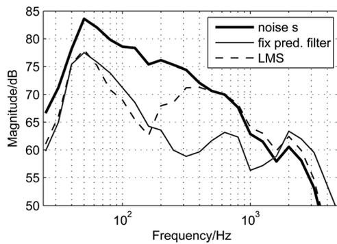
**Fig. 15** Measurement results from pink noise  $x$  and the residual noises after ANC
