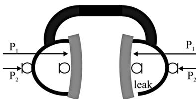
**Fig. 2** Measurement of the passive attenuation  $P = (P_{in}/P_{out})$  in a tight case on the left and a leaky case on the right
