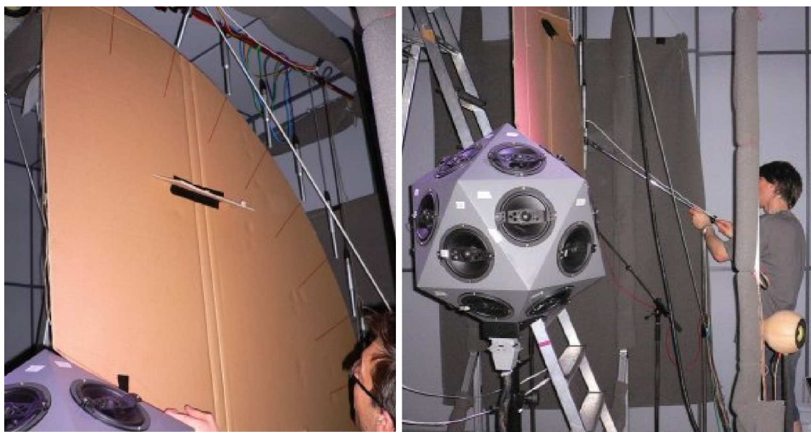
Figure 5: Adjusting the circular array microphones. We disregarded the axial aiming of the microphones.
