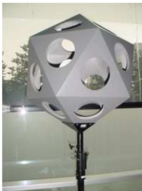
Figure 1: The icosahedral skeleton for the loudspeaker array in February 2006.
