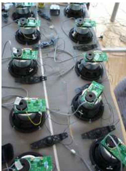
Figure 2: Joining the cross-over circuits with the speaker drivers in April 2006.
